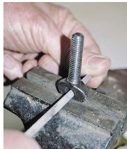
Use a slim triangular file to make the hexagonal hole for the Allen wrench.
