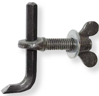
Here the blade and holder are ready to be fitted into the plane body.
