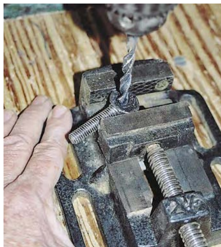
Drill the thumbscrew with a \frac{5}{16} " drill, as shown here. Note that the position is \frac{1}{8} " closer to the thread side of the head.
